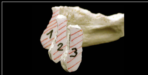
Sequential sectioning at 8 mm increments of sawbones
