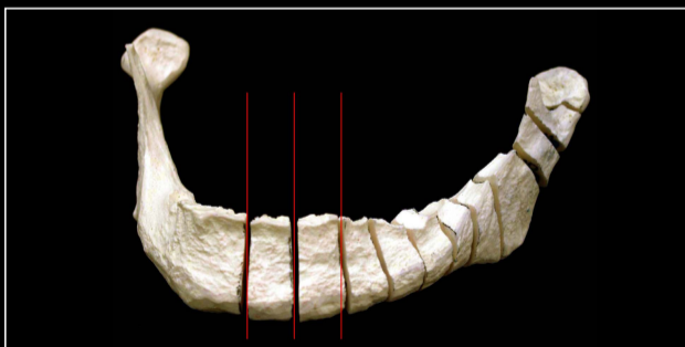
Sequential sectioning at 8 mm increments of sawbones
