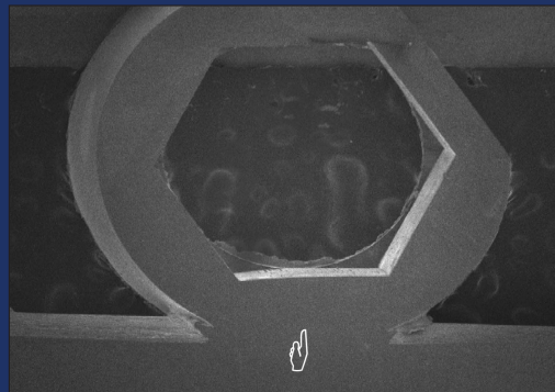
Fig. 4: Cross section of a welding joint at 20-fold magnification. Temporary abutment (round section above) and titanium bar (straight section below)
