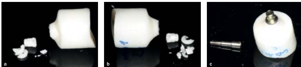
Figs 7a to 7c Types of failure of the abutments. (a) Prefabricated (SZ #4), (b) OP CAD/CAM (#3), (c) TP CAD/CAM (#3). Note the bent screw at the TP abutment.
