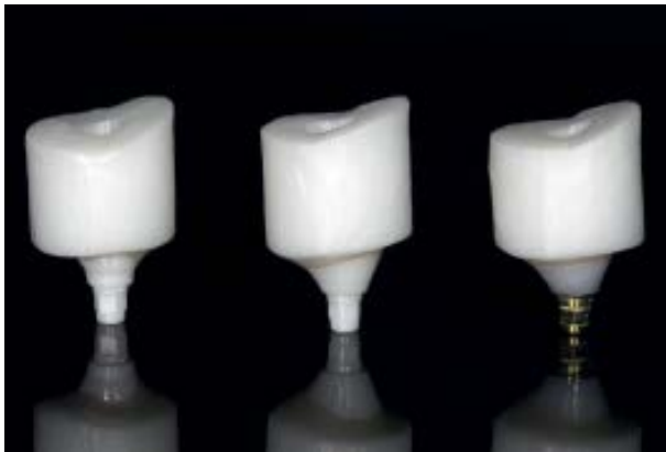
Fig 2 Simplified zirconia CAD/CAM crowns (CERCON) with 30-degree occlusal plane and occlusal screw access adhesively bonded to test abutments (left to right: SZ, OP, TP).
